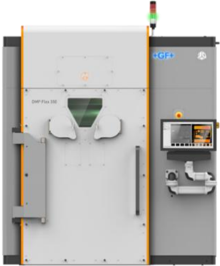
DMP Flex & Factory 350 max. Bauvolumen: 275 x 275 x 400mm (Single- oder Dual-Laser-Systeme)
